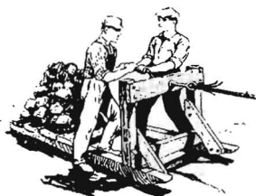
"Laying up" wire rope by hand. Weighted sled dragged forward as twisting proceeds.
