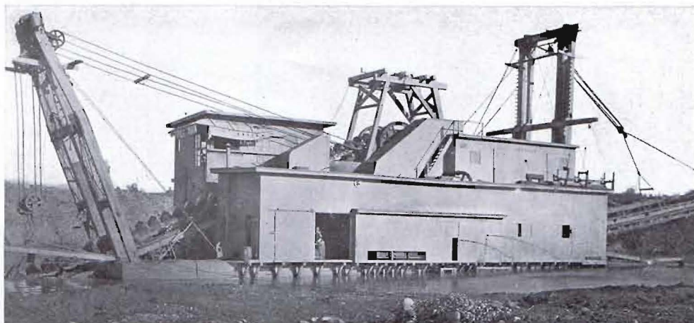
Complete view of Dredge, section of which is shown on Opposite Page. Carries 5460 feet of \frac{7}{8} -inch and 250 feet of 1\frac{1}{4} -inch Yellow Strand Powersteel Wire Rope.
